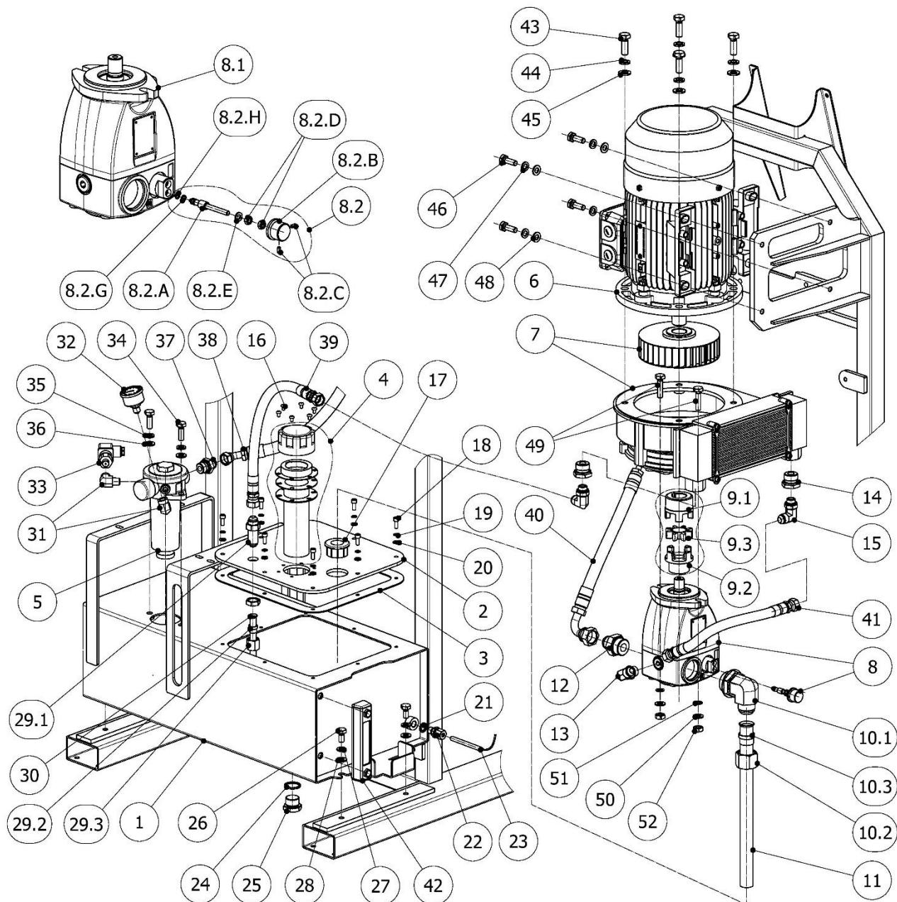
**Figure 3. Hydr. Power Unit 3PE~400V 50/60Hz, 4kW/5kW Motor (with 18/28cc Pump)**
