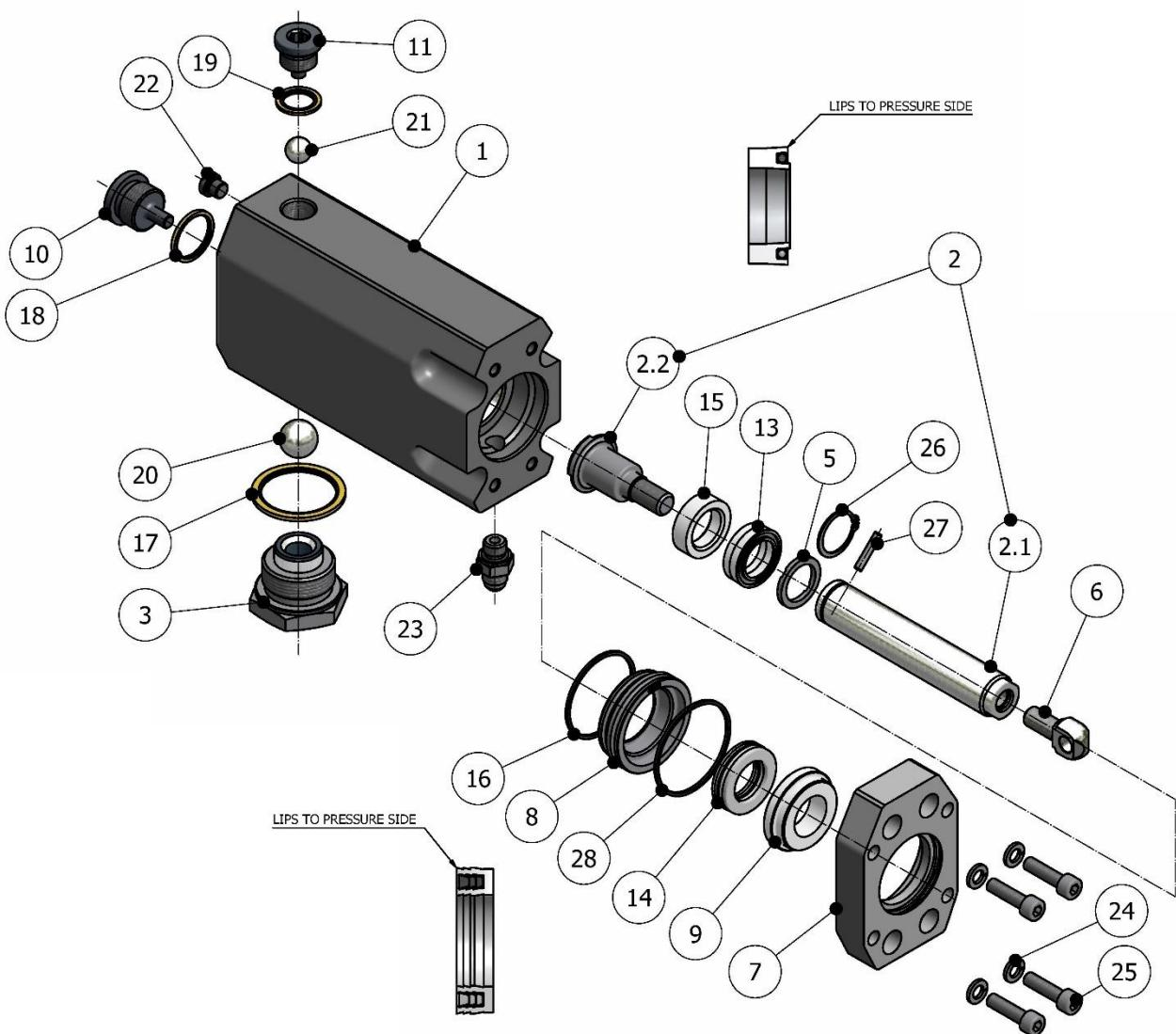
**Figure 10. "A" Proportioning Pump Assembly**
