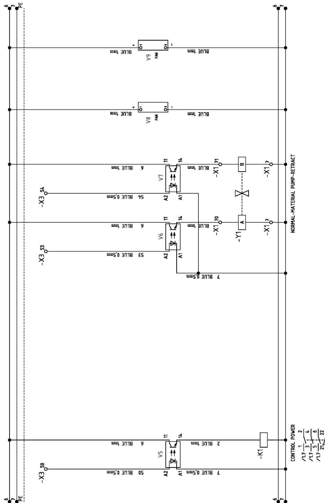
Figure 27. Elec. Schem. 3PE~400V 50/60Hz, “G-Connect+” (Sheet 2/7)
