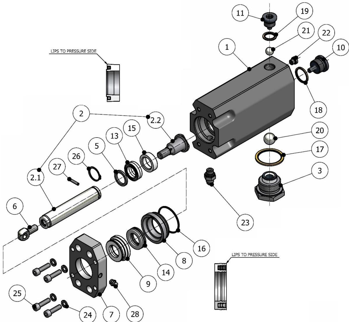
**Figure 11. "R" Proportioning Pump Assembly**
