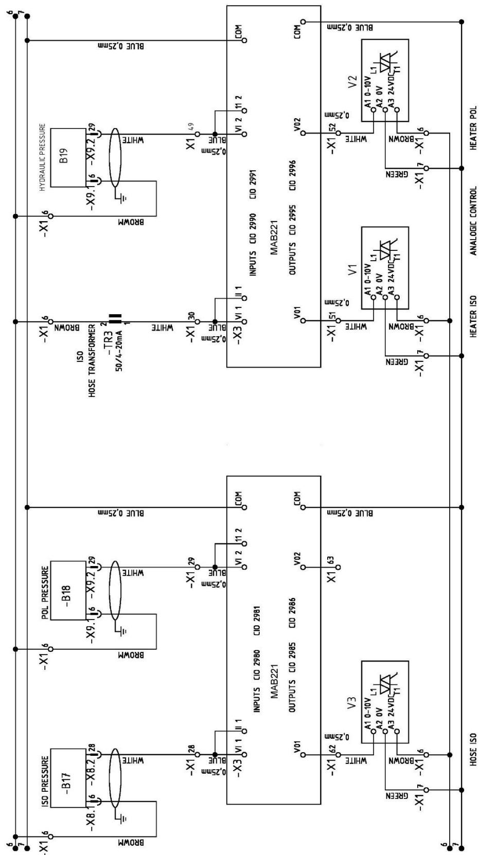
**Figure 30. Elec. Schem. 3PE~400V 50/60Hz, "G-Connect+" (Sheet 5/7)**
