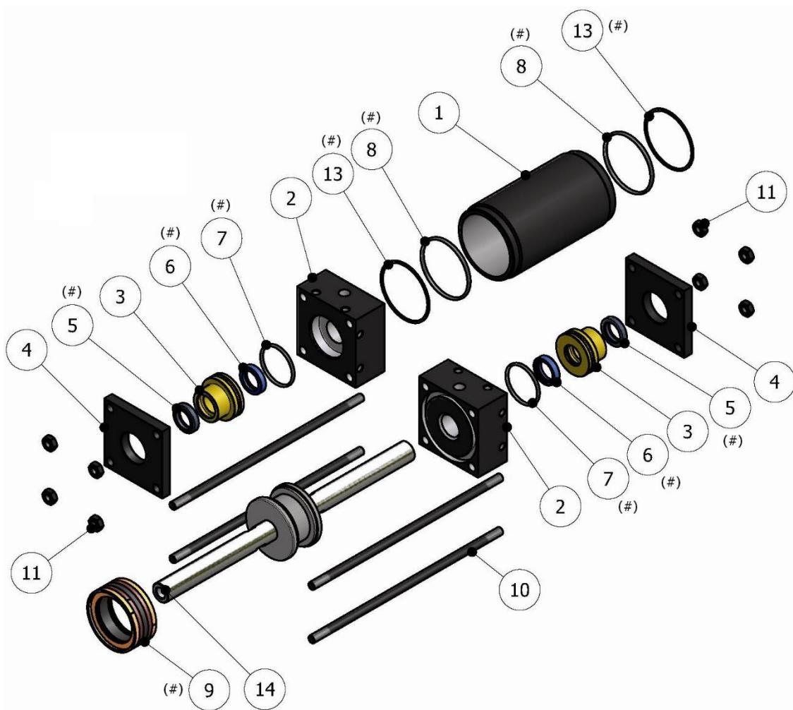
**Figure 9. Hydraulic Cylinder**
