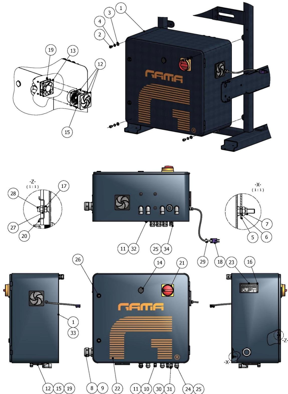
Figure 1. Electrical Component Cabinet, “G-Connect” and “G-Connect+”
