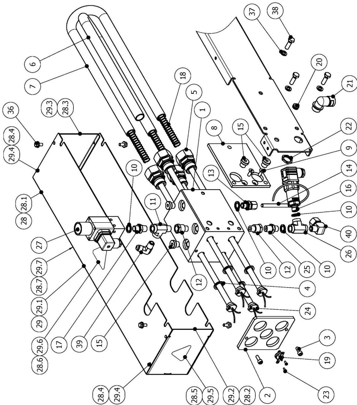
Figure 12. Primary Heater G-Connect
