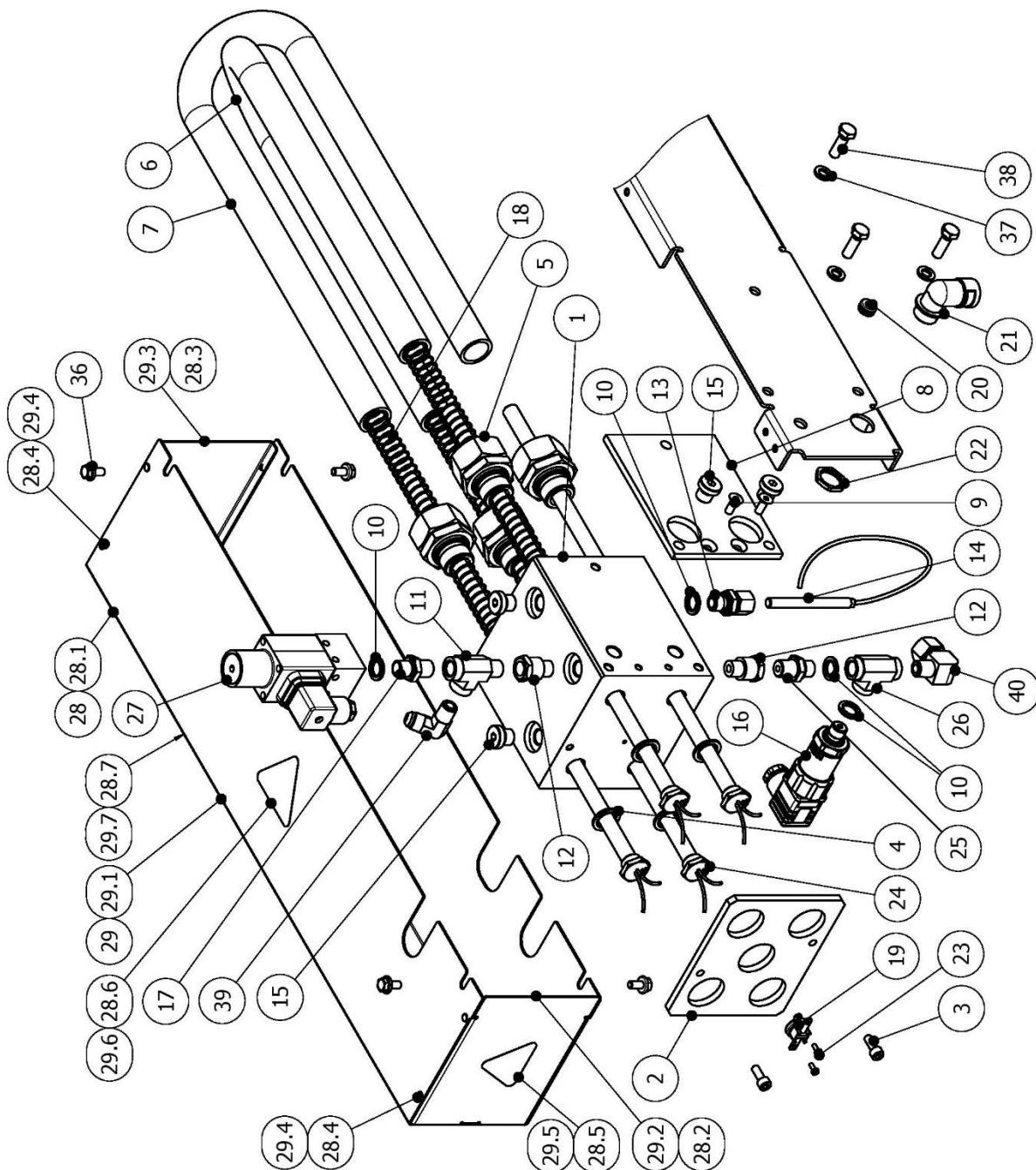
Figure 13. ISO and POL Primary Heater "G-Connect+"
